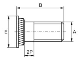
For plate thickness, min = 1.5 Head diameter E = 7 Hole diameter +0.1 = 6.4 Length B = 16 Male thread A = M4x0,7 Min distance to edge = 3.3
